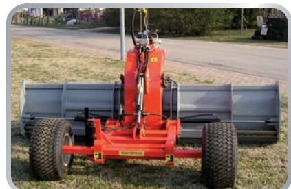
CON LARGHEZZA LAMA M. 2 ESTENSIBILE IDRAULICAMENTE FINO A M. 3
