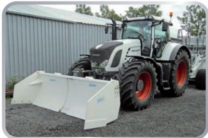
FRONT DOZER BLADE WITH FULLY HYDRAULICALLY CONTROLLED
